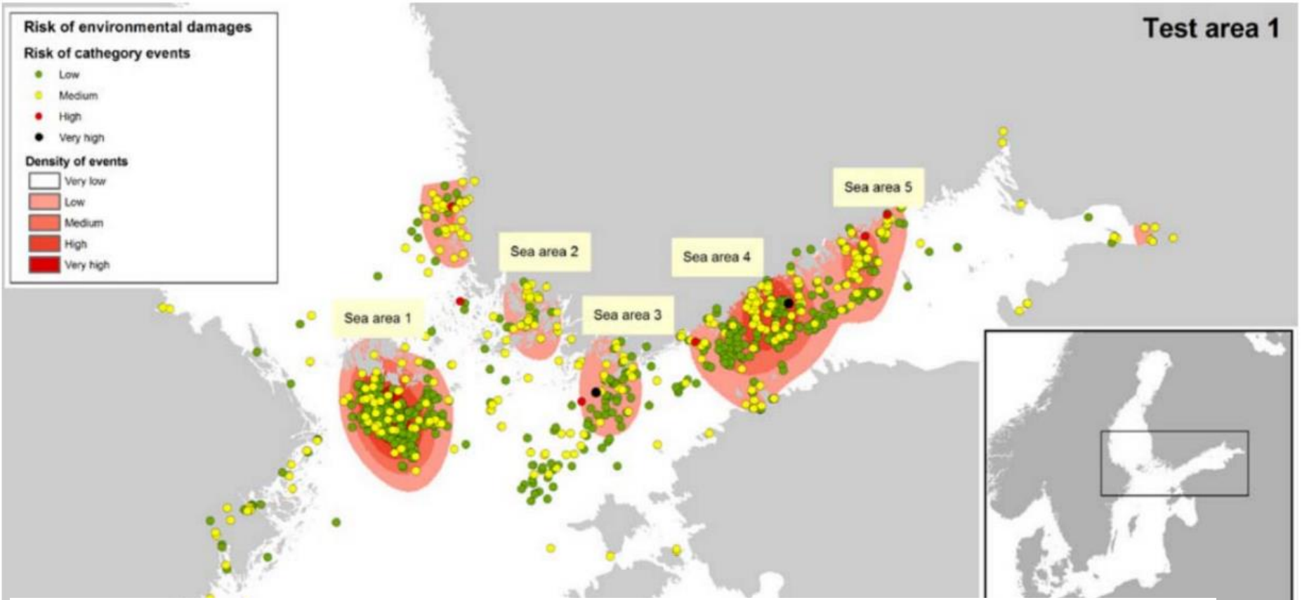
Kernel density GIS feature applied to incident statistics (with a total of 982 incidents registered from 2014-2016) for identification of accidental hotspot areas (OpenRisk, 2019).
